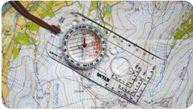
Photo 13 | Setting the map with the compass needle.
