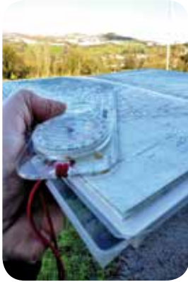
Photo 14 | Using line of sight with a set map. If you hold the compass on the map as shown, you can set the map with the needle, and sight along the edge of the base plate.
