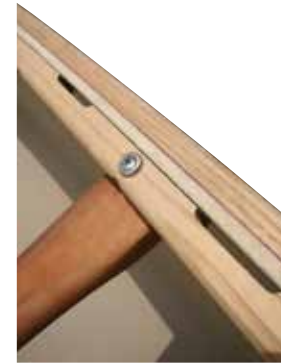
A Royalex canoe. Note the different layers of Royalex sandwiched between the wooden gunwales: two thinner layers of ABS on each side and an epoxy-soaked foam core.
