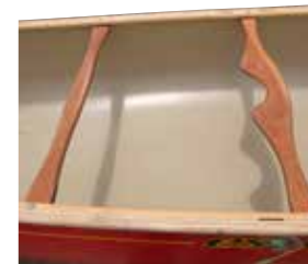
On the right is a carrying yoke; note the cut-out for your neck. On the left is a kneeling thwart.
